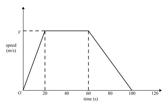
The car travelled 1.75 km in the 100 seconds.
