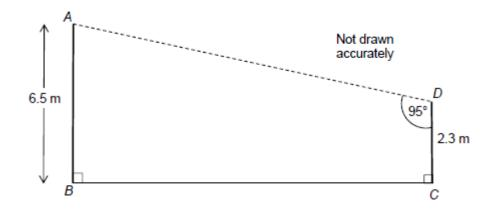
The zipwire will run between the top of two vertical posts, AB and CD. Work out the distance AD.
